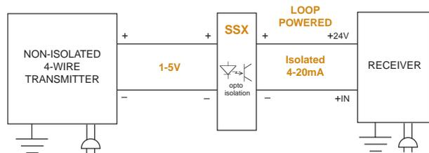
**Figure 5.** The SSX solves bucking power supplies. Also, when used with the -0HART option, the SSX acts as a current isolator that stops a HART signal from reaching a PLC, DCS or other receiving device.
